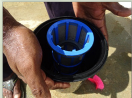
Reassembly of filter
