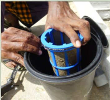
Removal of filter
